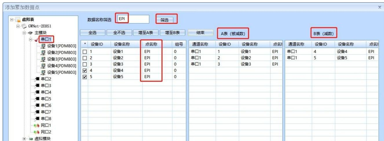
The dialog shows the 'Add Accumulation Data Point' configuration for 'Serial Port 1'. It includes a tree view of the virtual module, a search bar for 'EPI', and two tables: 'A表 (被减数)' and 'B表 (减数)'. The 'A表 (被减数)' table lists five devices with EPI values, and the 'B表 (减数)' table lists two devices with EPI values.
